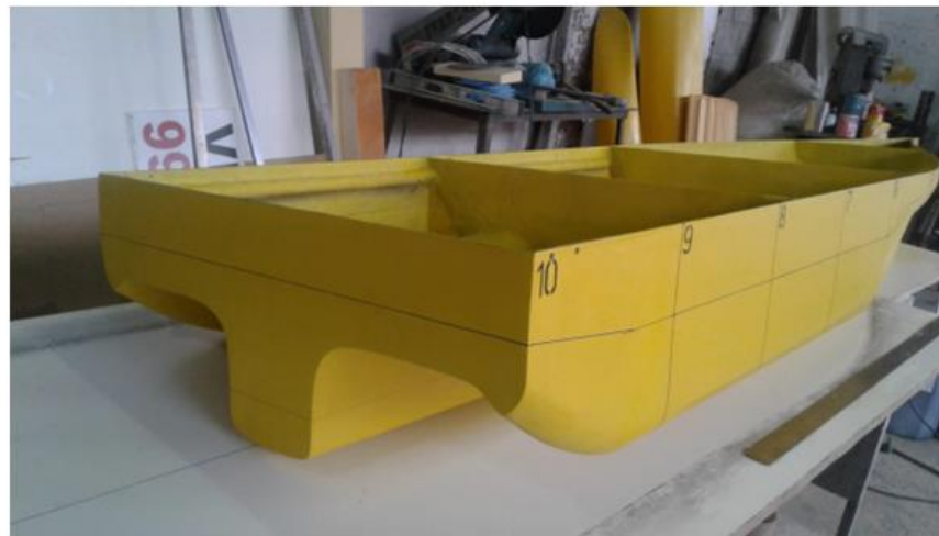
Figure 4 Model in the scale of 1:35 built in fiberglass.
