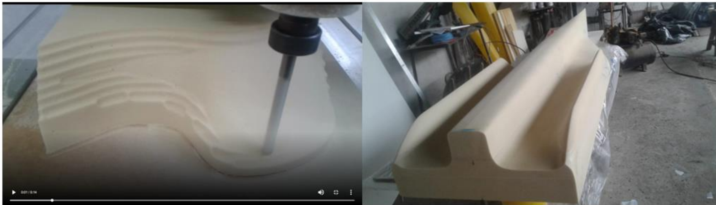
Figure 3 Mold in high density foam for building the model in fiberglass.
