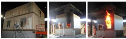
Figure 2 Wood-frame apartment fire test conducted at NRCC in Ottawa, Canada
