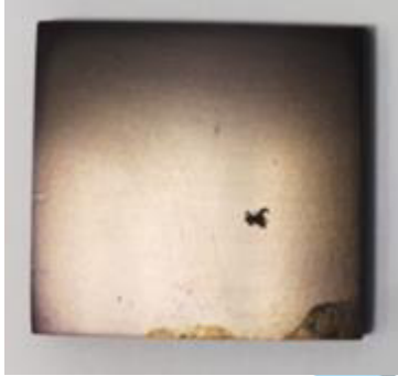
HAST: 130 °C and 95 % relative humidity without condensation
