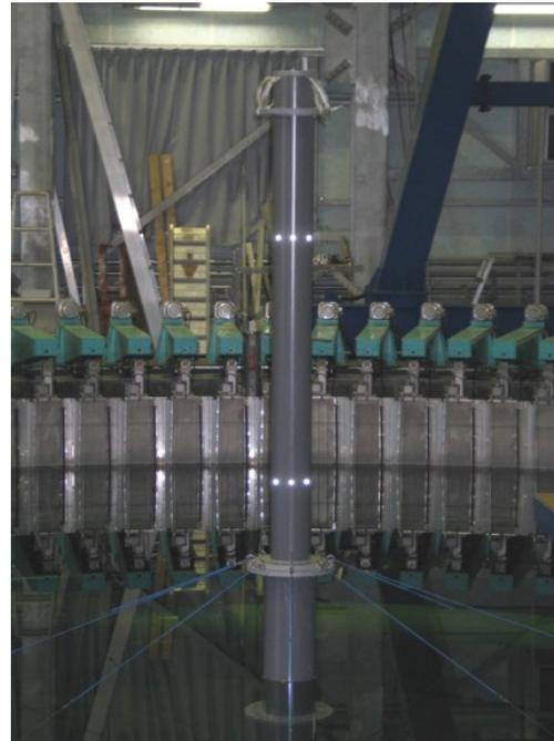
Hydrodynamic model Spar Buoy [NRMI - Japan]
