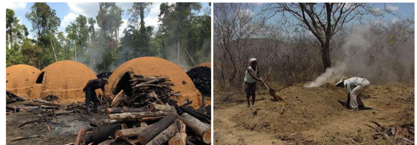
Fig 3. a) Half-orange kilns, the most used technology to produce charcoal in Brazil (6) . b) Charcoal production with a low efficiency technology for domestic use (7) .
