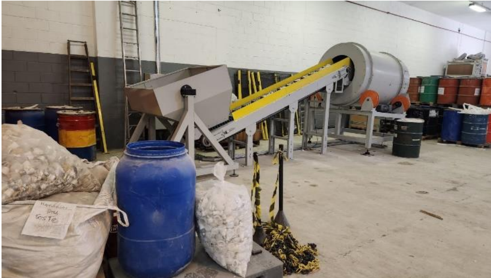
Autogenous mil applied on recycling of bulb LED lamps
