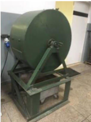
Tumbler parameters used as autogenous grinding
