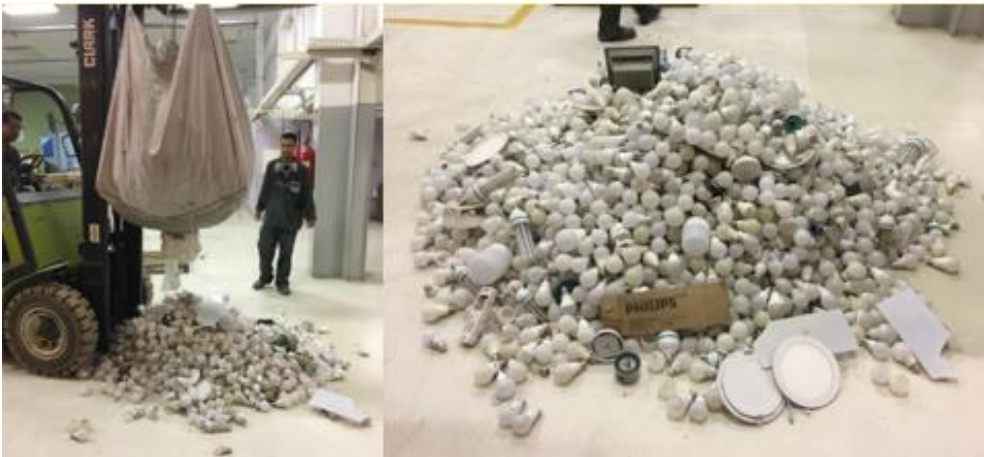
Construction of a conical stack for homogenizing the sample of LED lamps
