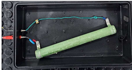
Fig. 2. Disruptive discharge simulator developed.
