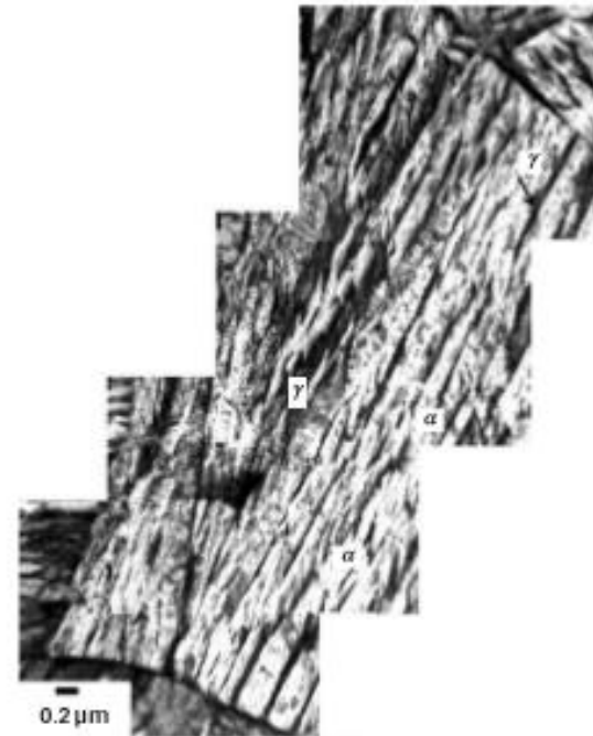
12.2 Transmission electron micrograph of carbide-free bainitic microstructure formed by air cooling after forging in Fe-0.30C-1.50Si-3.50Ni-1.44Cr-0.25Mo wt% steel. \alpha is bainitic ferrite and \gamma is austenite.
