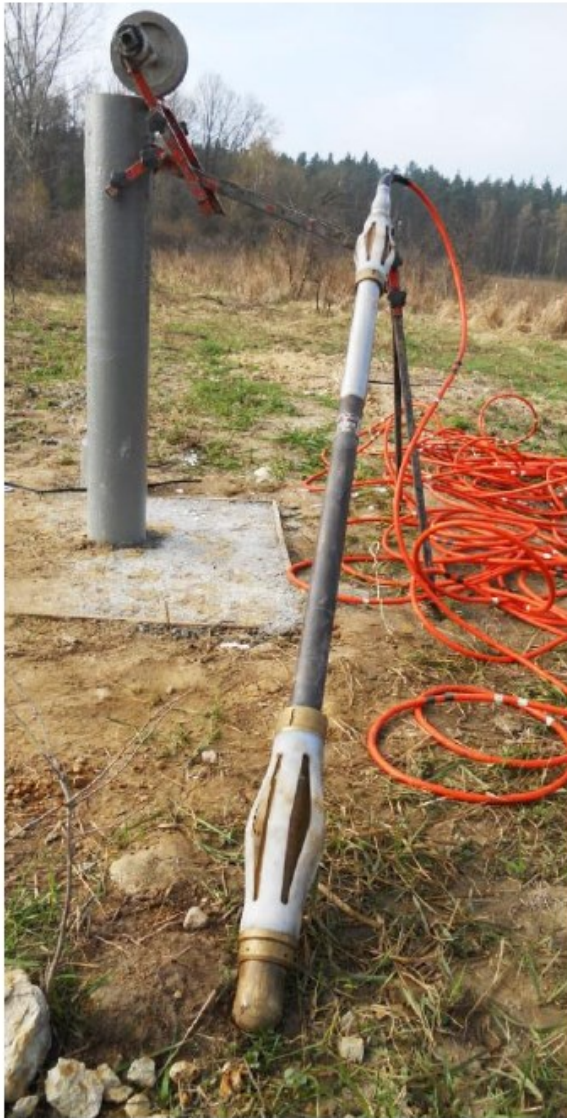
Figure 10, 11 – Inclinator Probe A15 (sx) and its Acquisition Unit (dx)
