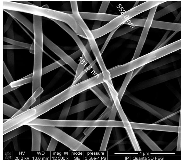
***PVA:active electrospun with a feed rate of 1.0 mL/h and tension of 12kV . SEM 12500x***
