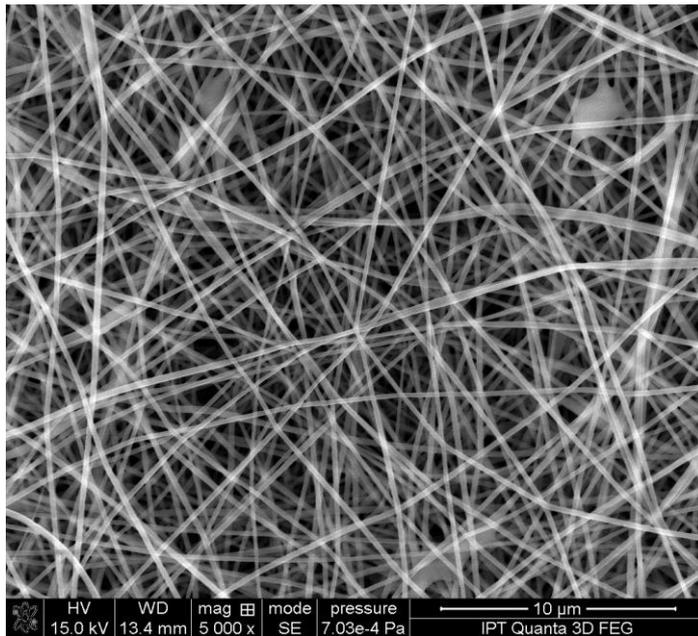
***PVP/PMMA electrospun with a feed rate of 1.7 mL/h and tension of 12.5kV . SEM 5000x***
