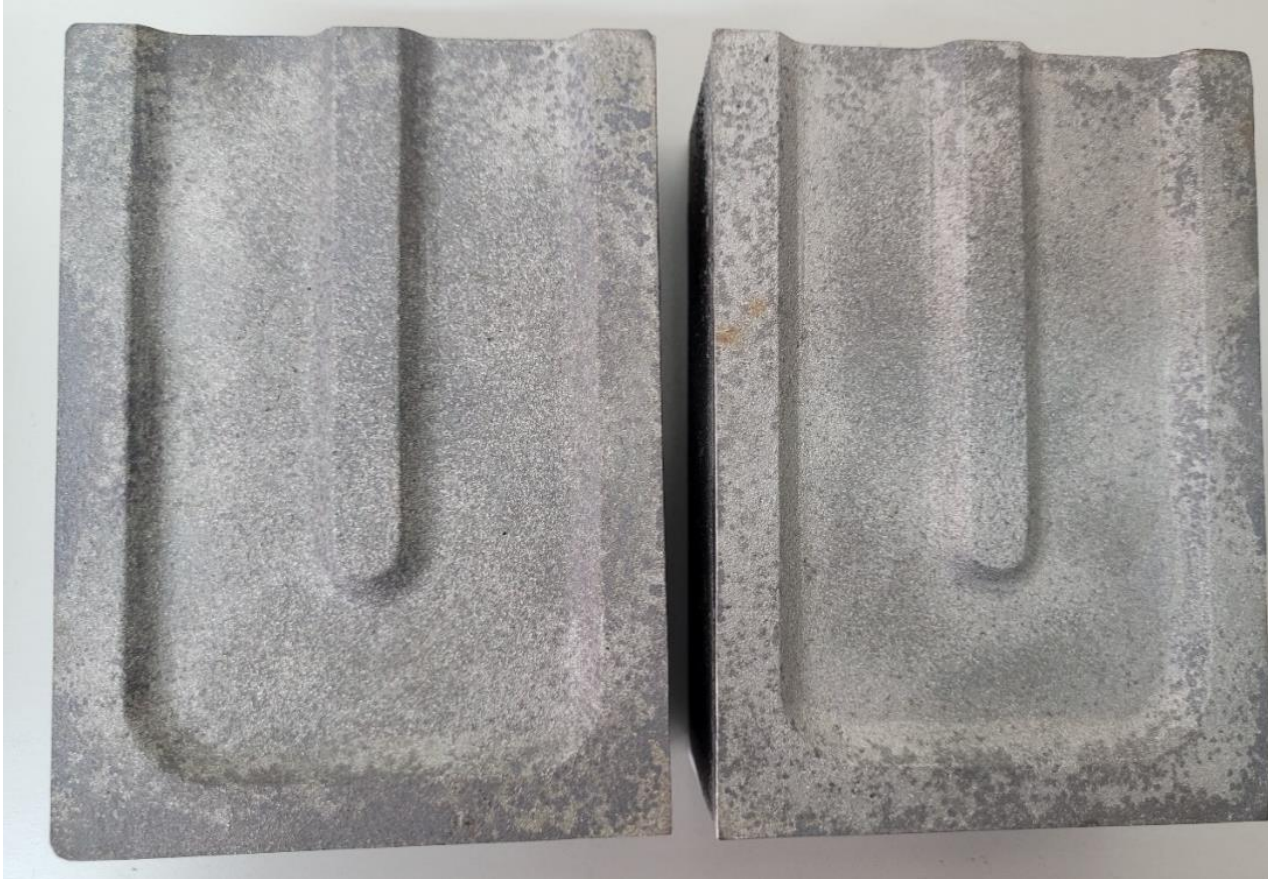
Test specimens for machinability tests
