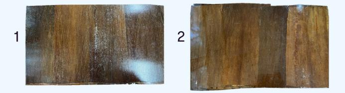
For density measurement, the results were  $0.79 \pm 0.04$  g/cm<sup>3</sup> (Material 1) and  $0.91 \pm 0.20$  g/cm<sup>3</sup> (Material 2). Lower density values are advantageous for polymer composites as they indicate the potential for lighter materials. The moisture content results were 5.30 ± 0.30% (Material 1) and 4.90 ± 0.60% (Material 2).
