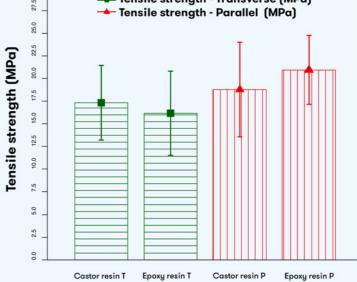
The results indicate a close resemblance in tensile strength values between composites with tururi fibers arranged transversely: 17.33  $\pm$  4.12 MPa (Material 1) and 16.18  $\pm$  4.65 MPa (Material 2). Comparable values were observed for composites with tururi fibers arranged in parallel: 18.78  $\pm$  5.22 MPa (Material 1)and 20.95  $\pm$  3.80 MPa (Material 2).
