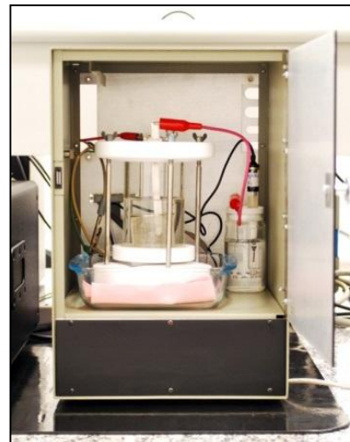
Experimental arrangement for electrochemical and galvanic corrosion tests
