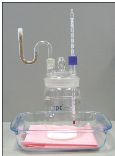
Test vessel used for the corrosion rate determination
