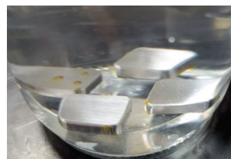
Test specimens in the flask after 1 hour – Localized corrosion points
