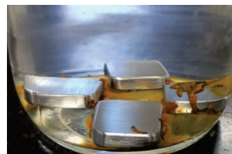
Test specimens in the test bottle after 24 h – Corrosion caused by the crack
